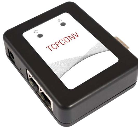
TCPConv adds a device, which is equipped with a USB- or RS232-interface into your local area network (LAN). A typical application is the extension of a network device (i.e. a network printer) by a local peripheral device. Simply insert TCPConv into the existing LAN connection of your device. In order to do so, TCPConv contains 2 LAN ports, which operate as a network switch.
