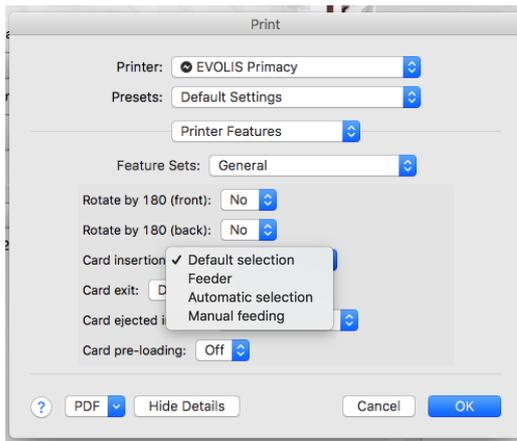
**Default selection:** recommended setting according to the type of current printer
