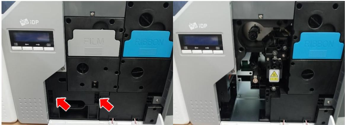
*Figure 39 Remove module (IC, RF)*
