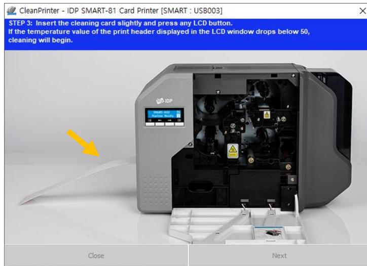
*Figure 90 Printer cleaning step 3*
