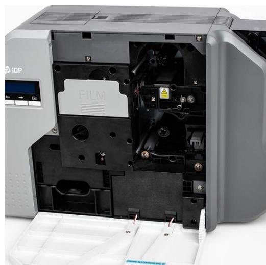
*Figure 16 Installing film cartridge*
