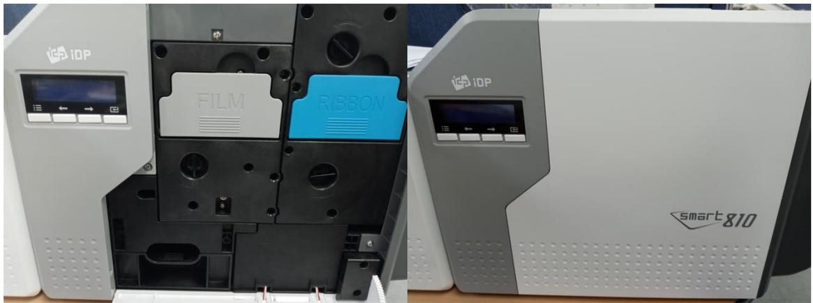
*Figure 41 Install module (IC, RF) 3*
