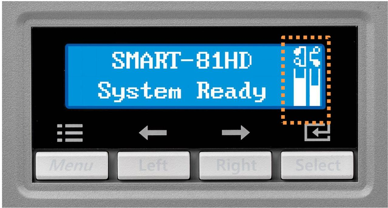
*Figure 6 SMART-81 Display and Buttons*
