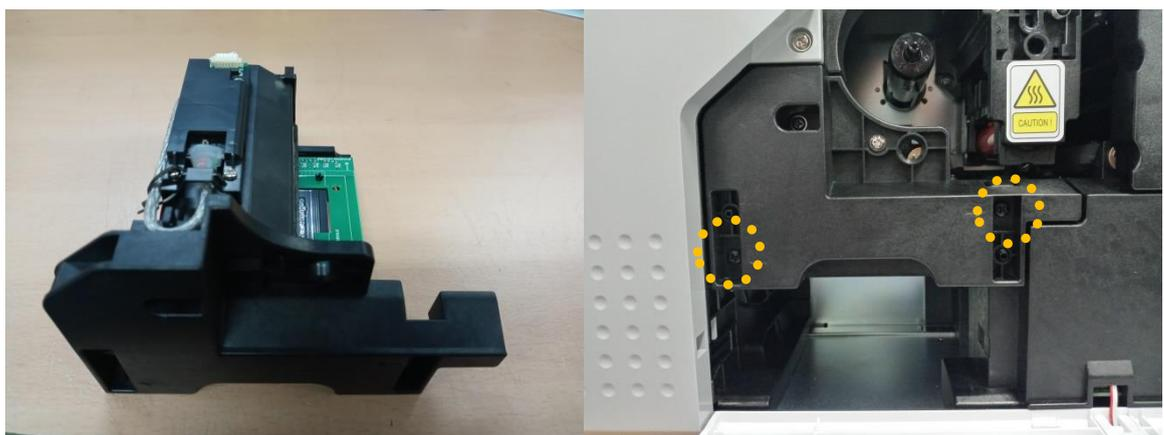
*Figure 40 Remove module (IC, RF) 2*
