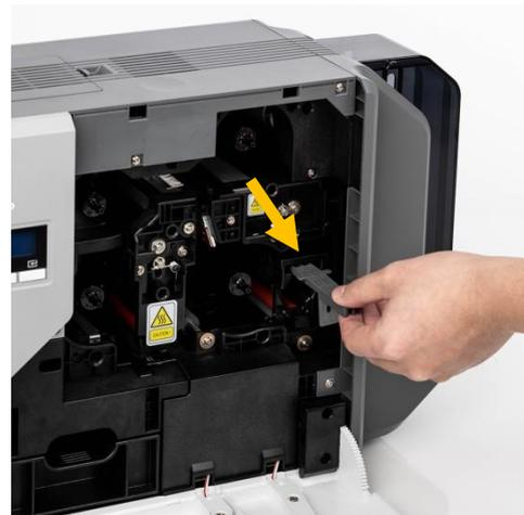
*Figure 11 Take out cleaning roller Cartridge*
