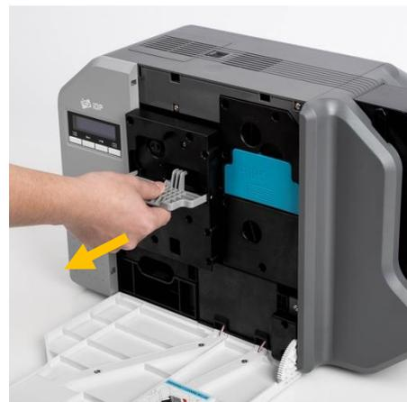
*Figure 9 Remove film cartridge*
