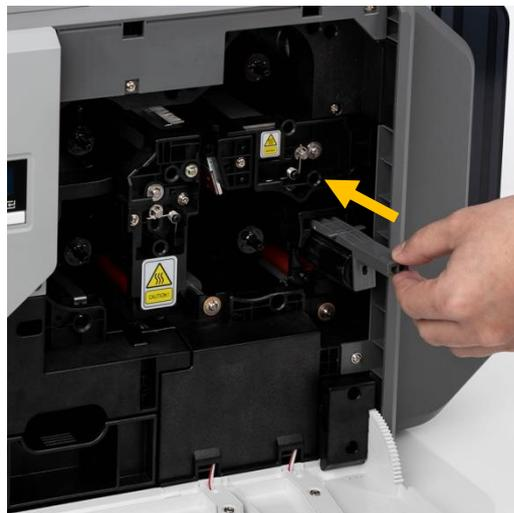
*Figure 15 Installing the cleaning roller cartridge*
