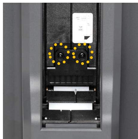
*Figure 21 Adjusting card thickness lever*
