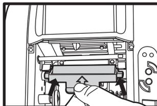
Place roller assembly back into printer
