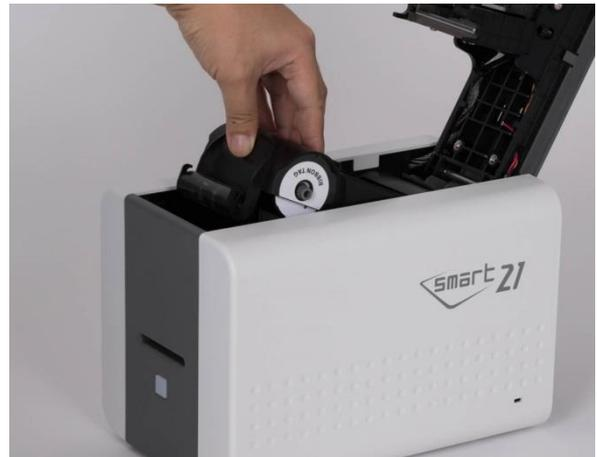
*Figure 15 Installing the ribbon cartridge*
