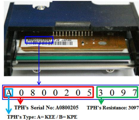
Figure 67 Thermal Print Head
