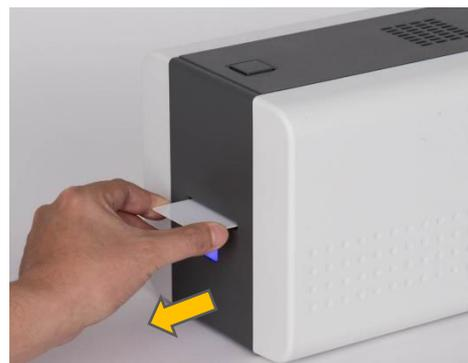
Figure 19 Unloading the card
