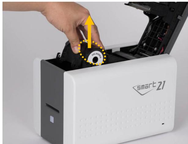
*Figure 10 Take out the ribbon cartridge*
