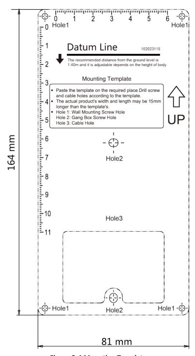
**Figure 3-4 Mounting Template**
