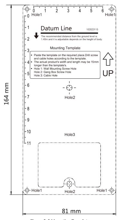
**Figure 3-6 Mounting Template**
