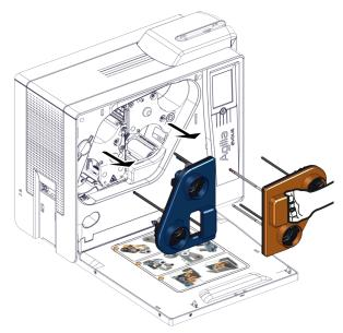
6. Remove the printing ribbon and retransfer film from the cassettes. ("Replacing a printing ribbon or retransfer film" on page 39).
