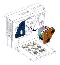
1. Open the door of the printer and remove the orange cassette.
