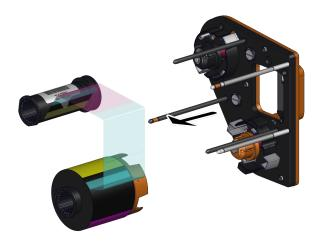
2. Remove the ribbon from the cassette. <u>"Replacing a</u> printing ribbon or retransfer film" on page 39
